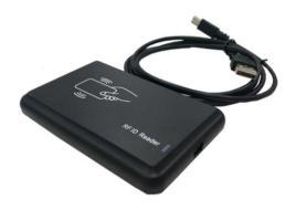
KB581 dual-frequency card reader is a two-in-one card dispenser, it can read LF 125KHz EM4100 card as well as HF 13.56MHz Mifare card. It adopts USB non-drive technology, plug in and play. And the analog keyboard greatly improves the speed of entering card data.
