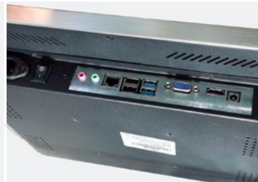
4 USB, 1 audio in & out, 1 HDMI, 1VGA, 1 Lan, 1 parallel
